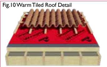
Fig. 10 Warm Tiled Roof Detail Wraptite fully adhered to substructure with min. 11mm counterbattens.
