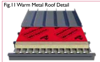
Fig. 11 Warm Metal Roof Detail Wraptite fully adhered to substructure. Metal sheet installed according to manufacturer.
