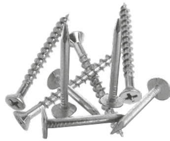
Screws and Nails 30mm screw or nail for tile fitment 50mm screw or nail for ridge/hip cap fitment 75mm to 80mm screw or nail for RidgeMaster/ HipMaster fitment
