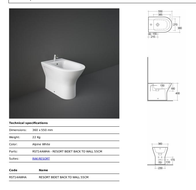
Dimensions: All dimensions in mm. Tolerance of vitreous china & fireclay items:  $\pm$  5% for below 200mm and  $\pm$  3% for above 200mm; for all other items tolerance  $\pm$  1%. Note: Due to a continuing development program to improve design and performance, the manufacturer reserves all rights to vary specifications without prior information. Please note accessories are for photographic use only.
