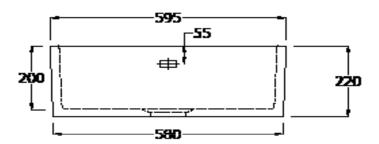
Dimensions: All measurements are in millimeters and are subject to normal manufacturing variations.
