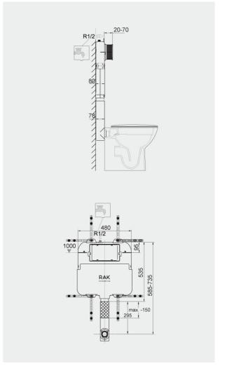
Dimensions: All dimensions in mm. Tolerance of vitreous china & fireclay items:  $\pm$  5% for below 200mm and  $\pm$  3% for above 200mm; for all other items tolerance  $\pm$  1%. Note: Due to a continuing development program to improve design and performance, the manufacturer reserves all rights to vary specifications without prior information. Please note accessories are for photographic use only.
