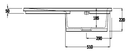
Dimensions: All measurements are in millimeters and are subject to normal manufacturing variations.
