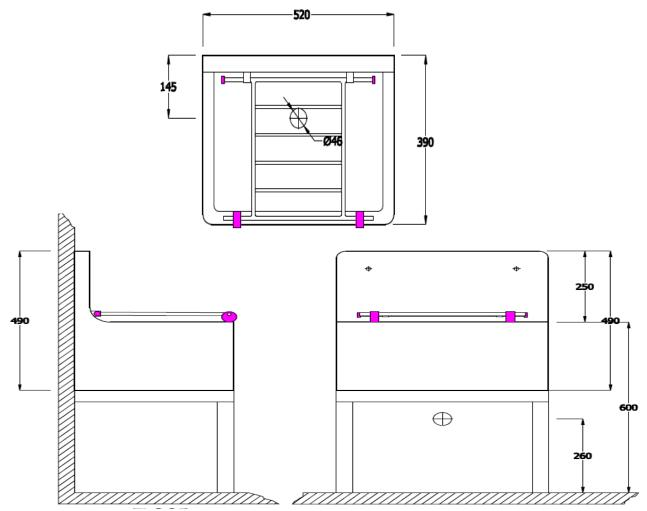
Dimensions: All measurements are in millimeters and are subject to normal manufacturing variations.
