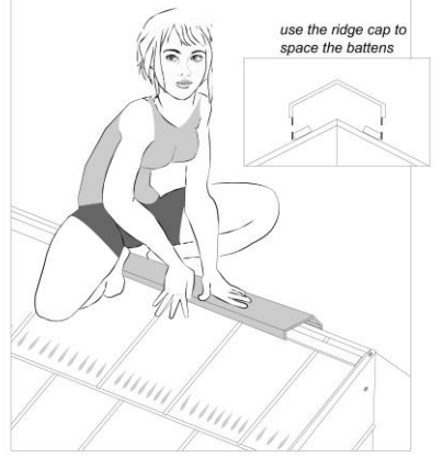
Attach Battens for Ridge Cap
