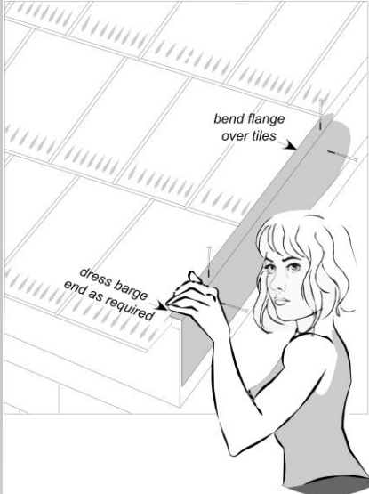
Attach 2 piece non handed barge board outer
